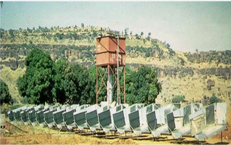
1966: Ormat's first solar powered unit of 600 W powering a water pump in Mali
